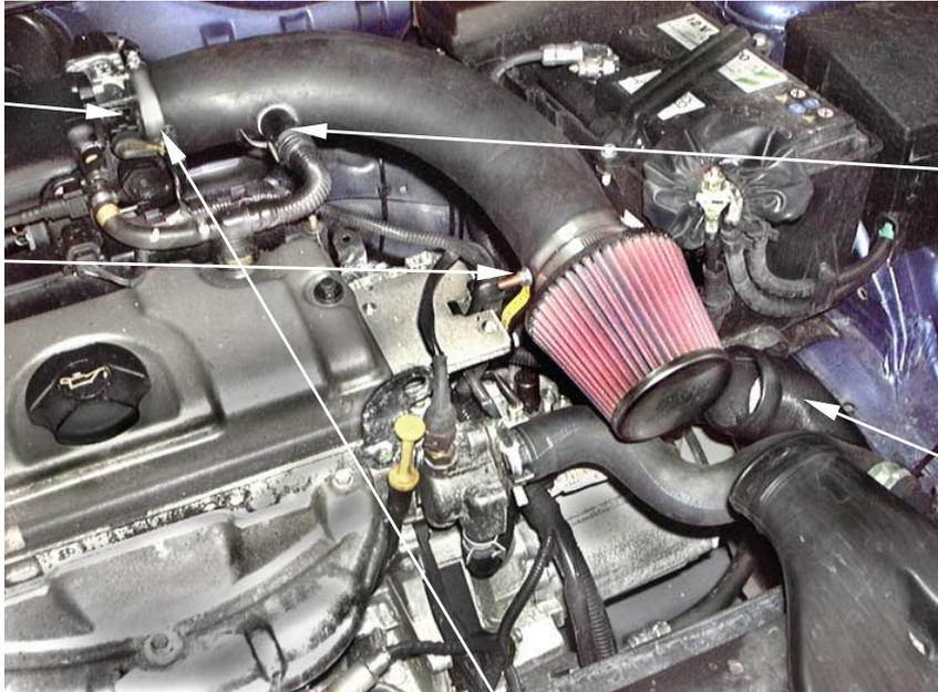
1. Fit the new rubber intake hose to the throttle housing, Do not fully tighten the clip.
