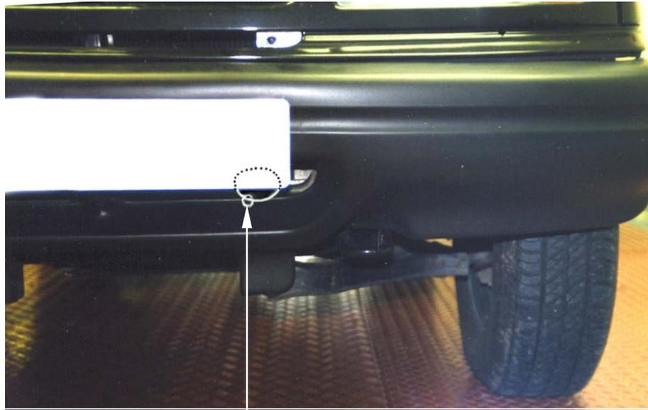
Feed the flexi cold air hose down towards the front L.H.S. lower grille, then pierce / drill a 3mm hole in the lower part of the bumper / grille and also in the end of the cold air hose. Attach the hose to the grille with the medium plastic tie.
