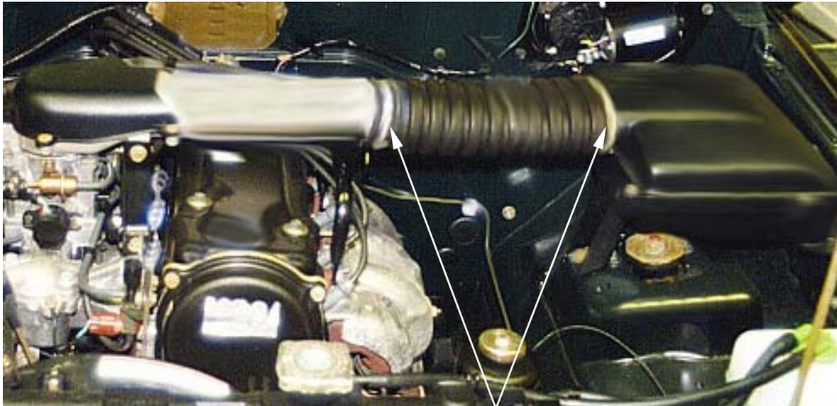
Unclip and remove the rubber intake hose leaving the air box in place.
