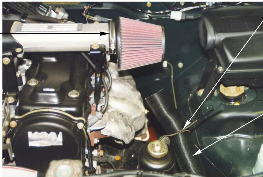
2. Lengthen the flexi cold air hose to 32" / 81cm. Tie the flexi cold air hose to the PAS hose coming from the reservoir with the long plastic tie supplied.
