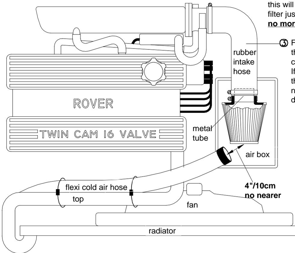
③ Fit the filter assembly to the longer end of the new rubber intake hose and fit the complete assembly to the intake manifold. If necessary pull the two breather hoses on the throttle body back 3mm to allow the new intake hose to fit squarely. Do not disconnect the breather hoses.
