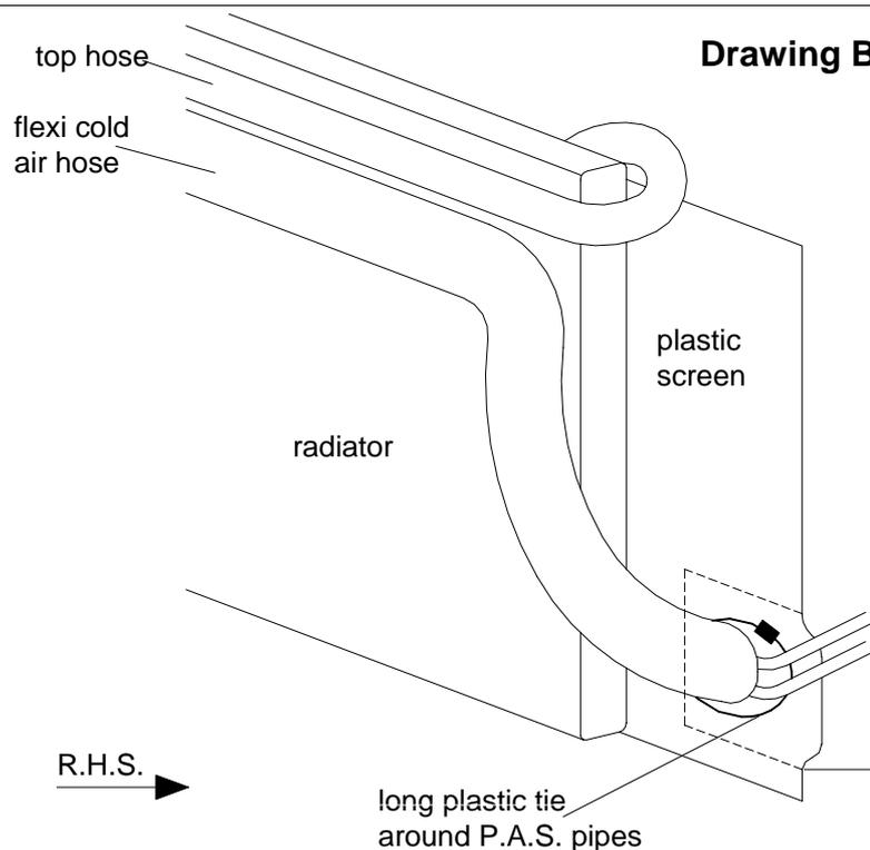
③ Attach the top hose to the P.A.S. pipe with a long plastic tie supplied.
