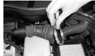
10. Install one of the supplied hose clamps onto the air intake tube.
