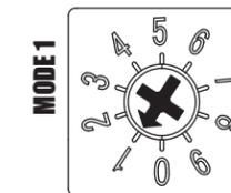
The Fatal Rev Limiter is to prevent catastrophic engine failure from missed shifts and broken drivetrain. This feature is adjustable from 400 RPM to 10,000 RPM. This rev limiter is always active, even when the 2 and 3 stage limiters are activated. When determining a value for the Fatal Rev Limit, consider the maximum RPM the engine can safely operate. The factory default setting for this feature is 5500 RPM.
