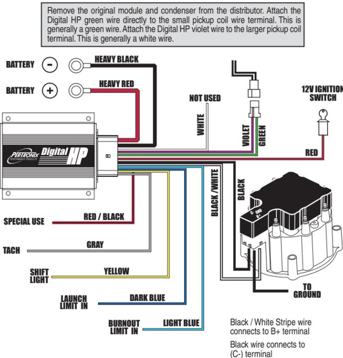
Remove the original module and condenser from the distributor. Attach the Digital HP green wire directly to the small pickup coil wire terminal. This is generally a green wire. Attach the Digital HP violet wire to the larger pickup coil terminal. This is generally a white wire.
