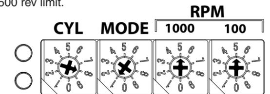
**Note:** Setting a rev limit values less than 1000 RPM requires that the "1000" switch be placed in the 0 position. For a maximum rev limit of 10,000 RPM both "1000" and "100" switches would be in the 0 position.
