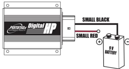
**Optional:** Programming of the Digital HP can be done before installing. This requires a 9V battery. Attach the small black wire to the battery negative terminal. Program your settings. When finished hold the small red wire on the battery positive terminal. The LEDs will blink indicating the setting is saved.
