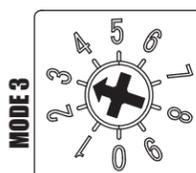
The Burnout Rev Limiter feature is only functional when the light blue wire is supplied 12V. Typically this is done with a momentary switch or toggle. The factory default setting for this feature is 3000 RPM.
