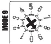
The trigger type, multiple spark and power settings are all set at the same time. Within this program mode, the Rev Limit Verification setting is also established (pg 15).
