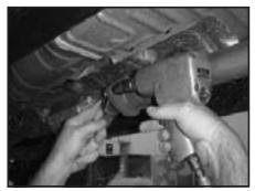
3. With the vehicle raised and properly supported, use the 14mm wrench, 14mm socket and ratchet to remove the bolts from the Catalytic Converter flange.
