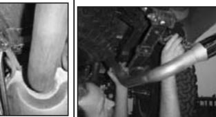
5. Using the pry bar, remove the tail pipe hangers from the rubber isolators.
