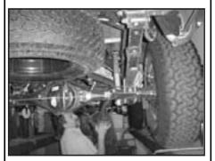
8. Remove factory exhaust from the vehicle.
