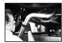
17. Install left-side axle pipe with hanger rod forward. Slip into muffler, mark to insure full insertion.
