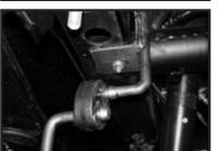
16. Install left-side rear frame bracket into existing hole in frame, behind tubular crossmember using hardware provided.
