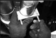
20. Install clamps at rear of muffler
