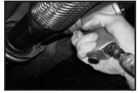
4. Remove nuts attaching muffler assembly, remove hanger rods from isolators, remove muffler assembly from
