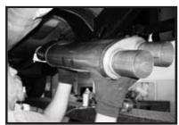
10. Install muffler onto intermediate pipe to insure full insertion. Align so tailpipes are flat
