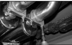
20. Finally tighten the support bracket.
