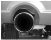
9. With the axle pipes in the muffler assemblies adjust mufflers to be flat, and the tips an equal distance from the bumper cover, Then tighten all clamps securely.
