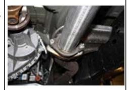
7. Slide one of the clamps over the inlet side of the rear Tip pipe. Slip the pipe onto the over axle pipe.
