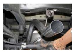
5. Slide one of the clamps over the muffler outlet then slip the muffler onto the over axle pipe and mount the muffler to the forward hanger on the frame. Do not tighten the clamp at this time.
