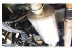
6. Slide one of the clamps over the muffler inlet then slip the New JBA intermediate pipe into the muffler inlet. Attach the JBA intermediate pipe to the stock y Pipe flange using the two supplied flange nuts. Do not tighten at this time
