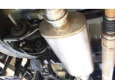
6. Slide one of the clamps over the muffler inlet then slip the New JBA S Shaped pipe into the muffler and the stock forward pipe.
