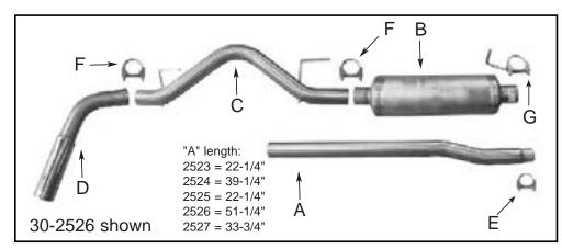
8. Slide the new JBA tail pipe with hangers (C) over the rear axle.
