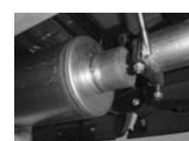
14. Insert Y Pipe into rear of the muffler.
