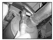
3. With the vehicle raised and properly supported, using the 15mm socket and ratchet, loosen the clamp, at the rear of the muffler, that secures the tail pipe to the muffler.
