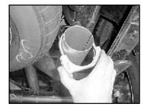
18. Install exhaust clamp (H) loosely over tail pipe (C). Do not tighten at this point.
