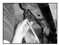
15. Insert rear tail pipe hanger into rubber isolator at the rear of the vehicle, near the spare tire.
