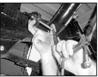
11. Install muffler hanger clamp (E) into rubber isolators near the rear of the factory muffler location.
