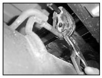
9. Remove muffler hangers from rubber isolators.
