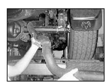
7. Remove tail pipe from the rear of the vehicle.
