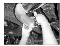
20. Position exhaust clamp (H) over exhaust tip (D).
