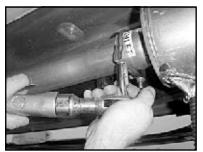
13. Insert muffler (B) into intermediate pipe (A). Place exhaust clamp with hanger(G) at the front of the muffler. NOTE: Support the muffler temporarily, until the muffler hanger clamp is used.
