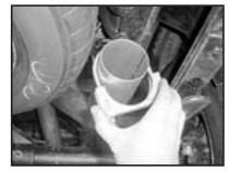
18. Install exhaust clamp (F) loosely over tail pipe (C). Do not tighten at this point.
