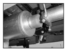
16. Insert tail pipe (C) through muffler hanger clamp (E) and into muffler (B).
