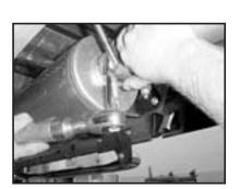
17. Align tail pipe (C) properly and tighten muffler hanger clamp (E).
