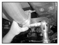
12. Install intermediate pipe (A) and secure with exhaust clamp (F).
