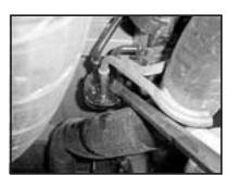
6. Remove the factory tail pipe hanger from rubber isolator.
