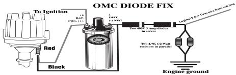
NOTE: Diodes and resistors connections should be sodered and insulated. The diodes and resistors can be found at most electronic stores. We recommend Digikey P/n's:
