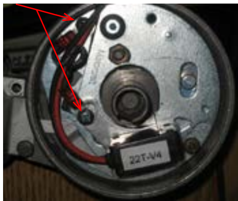
Ground Wire Location
