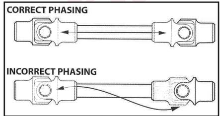
Sometimes if the u-joints are at a severe angle, even if they are phased correctly, a hard spot in the steering may occur for no apparent reason. If this happens, index the u-joints two or three splines in one direction. The hard spot should disappear or be minimized.
