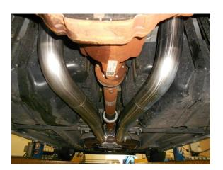
2) Place the left over-axle pipe **#26582H** into position over the rear axle and support with a stand. Then slide the front of the pipe into the clamp installed on the back of the factory H-pipe. Slide the pipe fully on and tighten the band clamp nuts enough to hold, but still allow for adjustment. Be sure that the over-axle pipe is fully forward. Repeat this step on the right side of the vehicle with pipe **#26583H**. See photos above.
