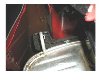
4) There are three hangers on each muffler, two in the front and one in the rear. Separate the rear hanger rods from the rubber mounts first, and then slide the mufflers forward and out of the front mounts. A spray lubricant will help the hangers to slip out. Then use a 13mm socket to remove the bolts securing the double hanger mounts at the front of each muffler from the frame on the left and right side of the vehicle. Place the mounts onto the front hangers of the corresponding Hurst muffler.
