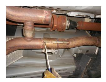
3) Use a 15mm socket to loosen the four nuts at the two band clamp connections at the rear of the factory H-pipe. Then using a screwdriver, pry up the clips on the clamp body to release the clip from the tab on the inlet pipes. Slip the over-axle pipes off and remove from the vehicle.
