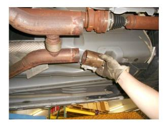
1) Remove the factory band clamps from the original over-axle pipes and place them onto the back of the factory H-pipe.
