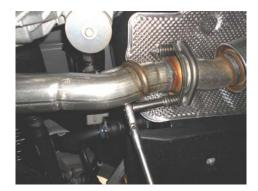
2) Using a 13mm socket, unbolt the left tailpipe assembly at the flanged connection at the rear of the muffler. Slide the three hanger rods out of the rubber mounts on the vehicle and remove the left tailpipe assembly.
