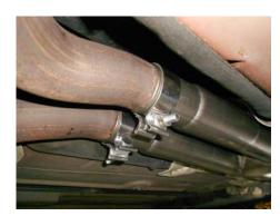
1) Begin the installation by placing a supplied 2-1/2" clamp onto each of the inlets of the X-pipe assembly **#26559H.** Then, place the X-pipe onto the back of the stock head pipes (the embossed Hurst H will be facing the ground). Level and center the assembly in the drive line tunnel and support with a stand. Tighten the two clamps enough to hold, but still allow for adjustment.
