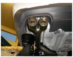
3) Place a supplied clamp onto the left muffler outlet. Place the left tailpipe #26564H into position and starting from the rear, connect the hangers on the tailpipe to the rubber mounts on the vehicle. Slide the tailpipe fully into the muffler outlet. Adjust the tailpipe so that the stainless tip is level and centered in the bumper cut-out. Tighten clamp enough to hold, but still allow for adjustment. Repeat this step for right tailpipe #26563H.
