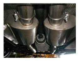
2) Place a supplied 3" clamp onto the inlet neck of both mufflers. Slide the mufflers onto the back of the Scavenger X-pipe assembly and support with stands. Level the mufflers and tighten the clamps enough to hold, but still allow for adjustment.
