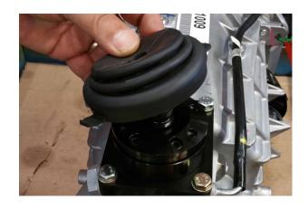
14. Install offset stick mount using supplied hardware.
