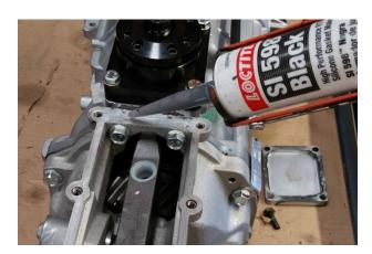
12. Install rear cover and bolt in place suing supplied hardware.
