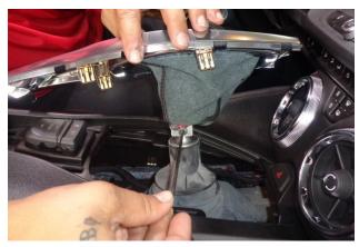
8. Align the screw holes on shifter handle and the stick. Start both flat head screws (2), then tighten them.
