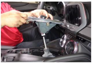
7. Install the handle body onto the shifter stick.
