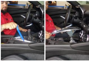
1. Use a plastic trim tool to separate the shifter bezel from the console, then lift the bezel straight up.
