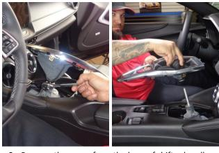
2. Remove the screw from the base of shifter handle, then lift the handle, boot and bezel off the stick.
