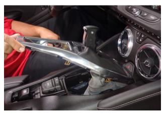
9. Reinstall the shifter bezel in the console.
