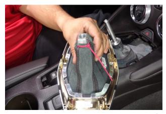
6. Use the supplied cable tie to secure the opening of the boot to the notch at the base of the shifter handle. Trim the excess cable tie.
