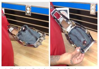
4. The plastic collar is glued to the shifter boot. Carefully separate the collar from the boot.
