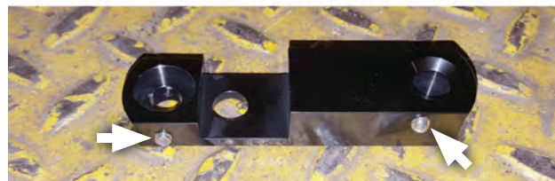
21. Thread (x3) set screws (21) almost fully into cable lever adapter (11) .
