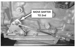
20. With the swivel still in the selector lever, move the shifter back through each gear position to SECOND, verifying that the swivel slips freely in and out of the lever in each position.
