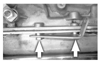
A. For stamped sheet-metal (stock) pans, use the two spacers between the pan and bracket.
