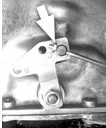
**18.** When the swivel slips freely in and out of the selector lever, snug the jam nut.
