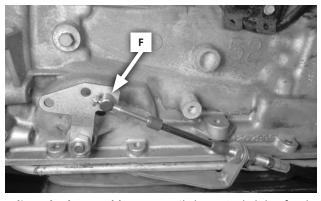
**17. Adjust the large cable nuts** until the swivel slides freely in and out of **hole F in the selector lever.** Gradually tighten the nuts against the bracket, while continuing to check the fit of the swivel in the selector lever.
