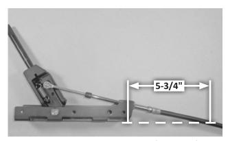
**6. Drill the cable hole.** Mark the center for the shifter cable hole 5-3/4" from the rear bend of the left shifter base. Move the shifter and cable out of the way, and drill or cut the 2" diameter cable hole through the floor.
