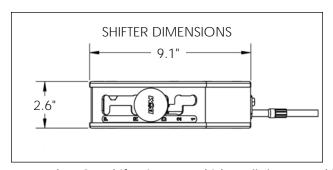
4. Locate the B&M shifter in your vehicle. Pull the carpet (if any) away from the floorboard where the shifter will be mounted. If the vehicle has a bench type seat, move the seat to the full forward position. Place the assembled shifter and cable on the floor, locating it for ease and convenience of operation. (Note the shifter dimensions, above.) The shifter cable must clear the front of the seat when the seat is in the full forward position, and the shifter grip must clear the dash
