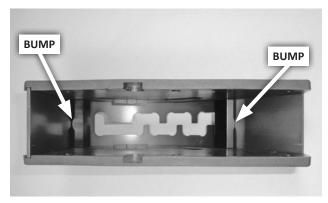
**CAUTION:** It may be necessary to loosen the top screws about a half turn, to allow the side covers to slip over the shifter base. If so, **ensure that the two spacers remain oriented correctly,** with the bumps touching the inside of the gate plate.
