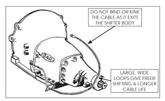
9. Route the cable approximately as shown. Avoid any sharp bends which may kink or otherwise damage the cable. Seal the cable hole shut to keep exhaust fumes, water, etc. out of the passenger compartment. Use clamps and/or cable ties (customer supplied) to secure the cable housing in such a way as to prevent contact with the exhaust system, engine, or any moving parts.
