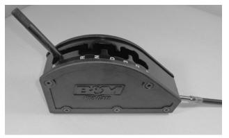
**10.** Ensure there is no debris in the shifter mechanism, then reinstall the assembled gate plate and side covers on the shifter base, using 3 screws along each side.
