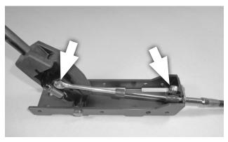
3. Assemble the shifter and cable. At the front (eye-end) of the cable, pull the two plastic dust boots all the way forward. Insert the cable through the notch in the shifter body. Secure the cable eye to the shifter pin with the E-clip. Then secure the cable housing tab to the shifter base with the 1/4-20 × 5/8" bolt and lock nut. Finally, push both plastic dust boots back over their respective joints.
