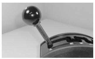
**11. Reinstall the jam nut (flats down) and shift knob.** Orient the knob as desired, then tighten the jam nut.
