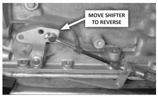
**19.** With the swivel still in the selector lever, move the shifter into REVERSE. Verify that the swivel still slips freely in and out of the selector lever. If not, adjust the large cable nuts (and the swivel, if necessary), until it does.
