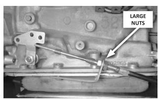
14. Attach the shifter cable to the cable bracket: First remove the small jam nut, two plastic dust boots, and one large nut and lock washer from the cable. Then insert the cable through the cable bracket, reinstall the lock washer and nut on the cable (loosely, to allow room for adjustment), and reinstall the two dust boots.
