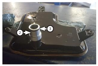
8. Fit **o-ring (3)** into groove on **extension (2)** then install onto transmission filter.
