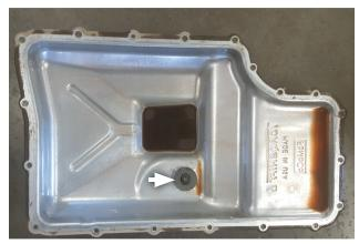
7. Remove and retain magnet from factory transmission pan.
