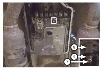
10. Fasten stock filter to transmission by installing screw (7) through washer (5), stock filter and spacer (8).
