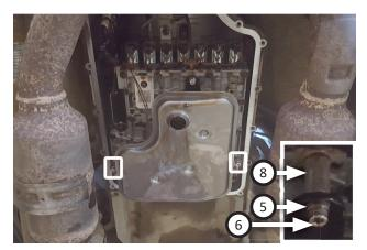
9. Fasten stock filter to transmission by installing (x2 ea.) screws (6) through washers (5), stock filter and spacers (8).
