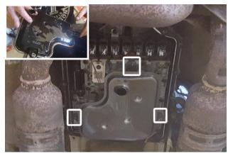
6. Remove (x3) bolts then pull transmission pan filter down and off of vehicle.
