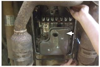
5. Remove and inspect transmission pan gasket. If it is still serviceable, clean and retain it, then wipe mounting surface.
