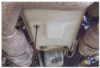
3. If possible, remove drain plug (your vehicle may not have a plug) and empty transmission fluid.
