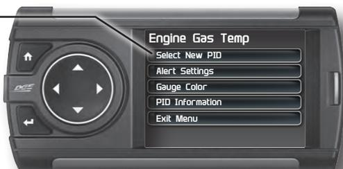
**STEP 4** - Use the Up/Down arrow buttons to highlight a new PID, then press Enter.
