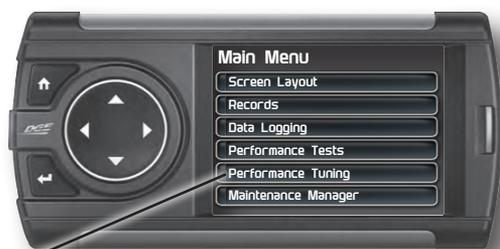
**STEP 3** - Use the Up/Down arrow buttons to scroll down to the Performance Tuning option. Press Enter.
