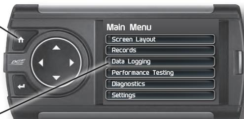
**STEP 2** - Use the Up/Down arrow buttons to scroll down to the Data Logging option. Press Enter.
