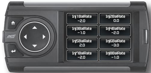
If you suspect a faulty injector, we recommend consulting a professional diesel mechanic who can verify the issue and also perform a cylinder power balance test to further diagnose.
