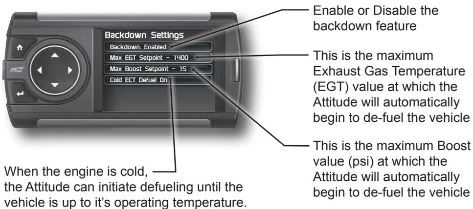
**CAUTION:** Other high performance modifications in addition to the Juice can allow the fueling to exceed the max set point and stock EGT levels, even after 100% de-fueling by the Attitude. This may result in detrimental EGT levels and potential power-train damage.
