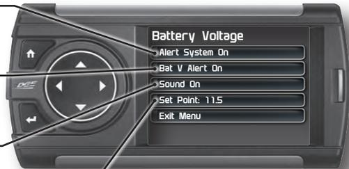
This is the point at which you want the alert to be triggered for this PID.
