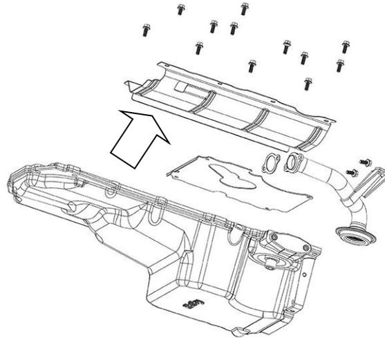
**IMPORTANT:** All gasket surfaces should be free of oil or other foreign material during assembly. Inspect the engine block oil gallery passages to make sure they are free from any debris or restrictions.
