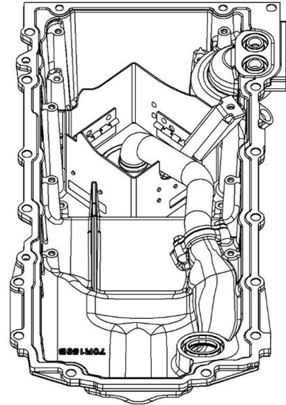
**IMPORTANT:** While the bolts are started, but still loose, lift the pickup tube. Tighten the two bolts while maintaining the lifted position. This process ensures proper clearance between the pickup inlet and the pan floor.
