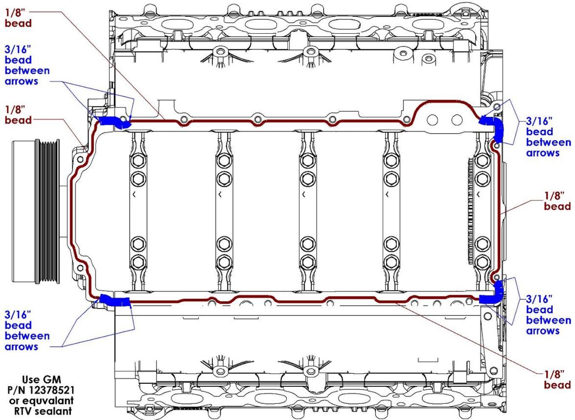
2. Apply a bead of RTV sealant (GM P/N 12378521 or equivalent) in the amount shown above.
