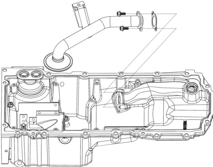
Install the oil screen/pickup tube and **gasket** with supplied (x2) M6 x 16 flange head bolts. Apply a drop of blue Loctite® to the threads before installing. You may need to slightly adjust the bracket to provide precise alignment of the hole. Torque the bolts to 10 ft./lbs.
