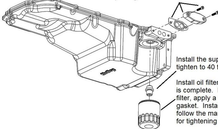
Install the supplied oil filter adapter and tighten to 40 ft./lbs.
