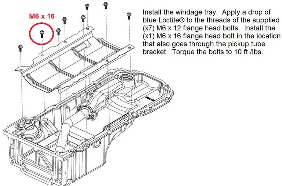
Install the windage tray. Apply a drop of blue Loctite® to the threads of the supplied (x7) M6 x 12 flange head bolts. Install the (x1) M6 x 16 flange head bolt in the location that also goes through the pickup tube bracket. Torque the bolts to 10 ft./lbs.
