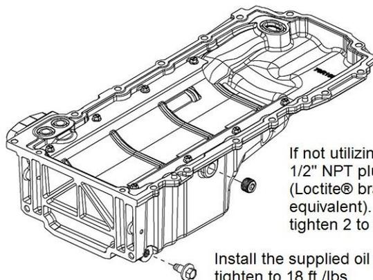
If not utilizing the oil return port, install the 1/2" NPT plug provided. Use thread sealant (Loctite® brand 567 pipe thread sealant or equivalent). Install to finger tight, then tighten 2 to 3 rounds.
