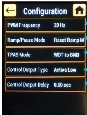
Change the frequency at which the solenoids are driven
