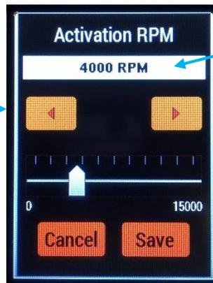
Adjust RPM via arrow buttons or manually enter RPM from 0-15000 RPM
