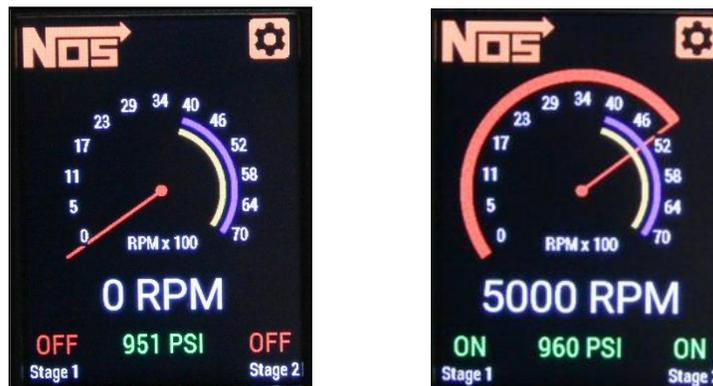
The bottle pressure display can be turned on or off in the dash setup menu. To allow for quick glances we've color coded the bottle pressure display as follows:
