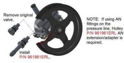
There are several pulleys that will fit the pump, but some do not have the correct belt alignment for this application. See applicable service manual for pulley installation procedures.
