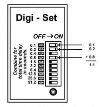
This time delay switch will allow you to activate a second stage of nitrous as a function of time.
