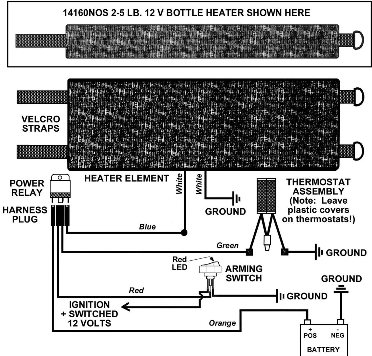
**IMPORTANT:** The heater should NEVER be operated without the thermostats in place. The thermostats MUST HAVE DIRECT CONTACT AGAINST THE BOTTLE SURFACE TO PROPERLY SENSE THE BOTTLE TEMPERATURE. THE PLASTIC COVERS MUST REMAIN ON THE THERMOSTATS!
