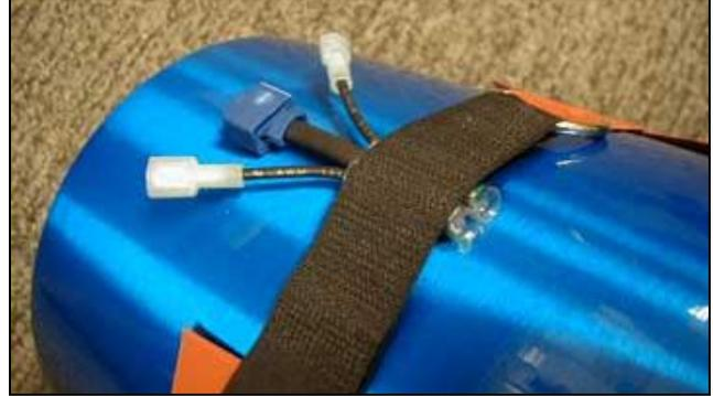
2. Secure the heater element around the bottle with the Velcro straps attached to the heater element.
