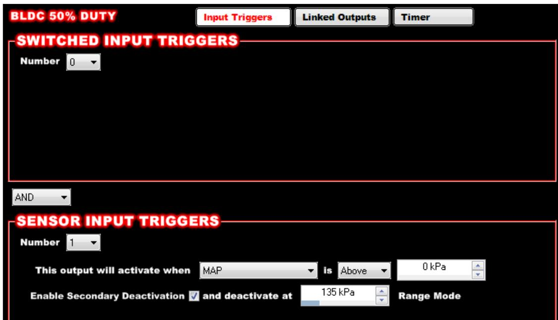
In this more advanced example, the pump would run at 50% duty cycle as long as:
