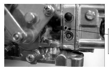
vacuum hose from this fitting to a vacuum source on the lower manifold.
