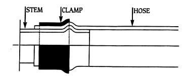
Slide clamp over top of fitting bead. Powergrip SB clamps have a wider sealing surface than conventional clamps and can be positioned over a wider area including the bead without causing leaks.
