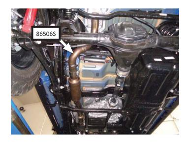
15. Place **clamp (MC250BS)** onto slip-fit of tailpipe. Connect tailpipe and rear inlet pipe then fasten mount to frame with bolts (x2) (removed step 4). Tighten clamp just enough to allow for adjustment.
