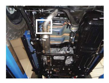
9. Loosen bolt on clamp at resonator inlet.
