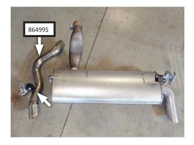
8. Remove stock resonator assembly from rubber isolator with a pry bar and retain for re-use.
