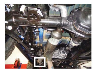
11. Remove clamp from resonator inlet and retain for reuse.
