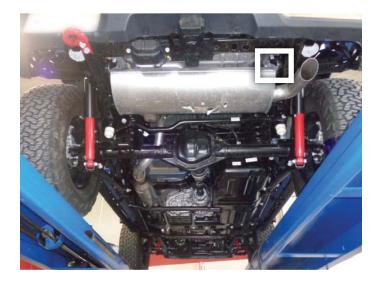
4. Remove bolts (x2) from mount on driver side above muffler in area indicated.
