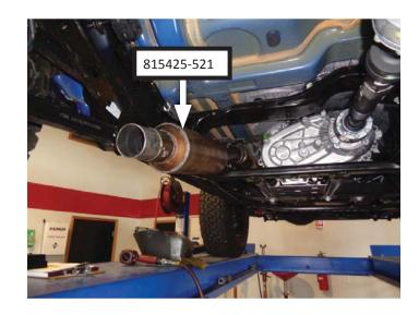
14. Place clamp (MC250BS) over muffler outlet. Place rear inlet pipe (86506S) into muffler with bend oriented over axle. Tighten clamp just enough to allow for adjustment.
