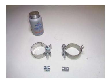
13. Place factory clamp (removed step 11) over ball end of factory inlet. Mate ball end of **muffler (815425-521)** to factory pipe and tighten factory clamp just enough to allow for adjustment.
