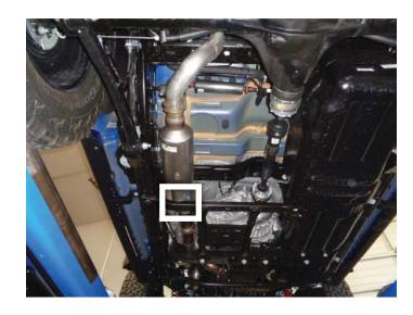
10. Rotate and remove resonator assembly from vehicle.
