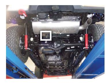
6. Remove muffler from vehicle.
