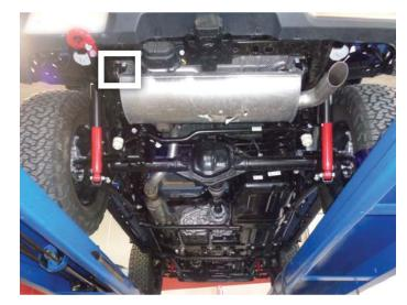
5. Loosen clamp at muffler inlet connection above rear axle.
