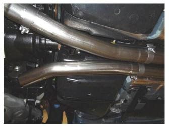
2) Place a provided 3.00" clamp onto the expanded end of left mid pipe #26702S, then slide completely onto the left side of the Scavenger assembly and tighten the clamp enough to hold, but still allow for adjustment. Repeat this step on the right side of the vehicle with mid pipe #26703S.
