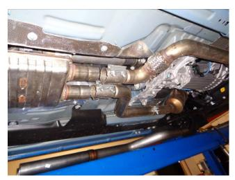
2) Support the center resonator with a stand; loosen the four nuts on the two band clamp connections at the resonator inlet. Slide the system to the rear to disengage from the clamps. See photos above.
