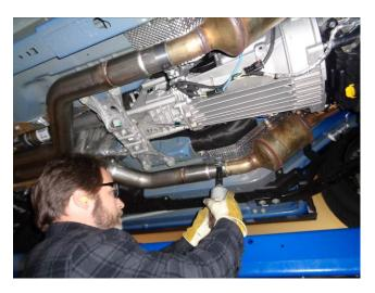
1) Place the provided 2.50" band clamps onto the front of the Scavenger assembly **26701S**, slide the assembly onto the factory head pipes approximately 3.00" and support the rear of the assembly with a stand. Be sure that the Scavenger assembly is centered in the driveline tunnel and that the embossed Flowmaster in the center case is facing the ground. Tighten both band clamps enough to hold, but still allow for adjustment.
