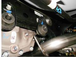
4) Place the right muffler assembly **#815430-487** up into position and slide the inlet completely onto the **26703S** mid pipe. Support the assembly with a stand and remount the rear hanger mount to the frame, tighten securely. Remount the front hanger to the cross member and tighten securely. Leave the clamp on the inlet loose for now. Repeat this step with muffler assembly **#815430-488** on the left side of the vehicle.
