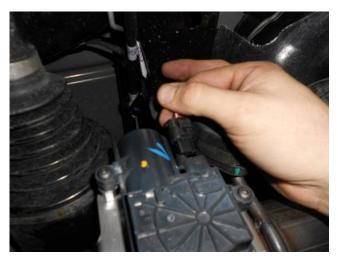
6) Reconnect the two electrical plugs removed in step 2 of the removal instructions back onto the tailpipe actuators now installed on the new Flowmaster tailpipes.
