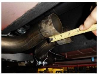
3) Begin the installation by placing a supplied 2-1/2" clamp onto each of the inlets of the Scavenger pipe **#26640S.** Then place the Scavenger pipe onto the back of the stock head pipes (the offset outlet pipe should be oriented to the passenger side). Level and center the assembly in the drive line tunnel and support with a stand. Scavenger pipe should slide over factory head pipe about 2". Tighten the two clamps enough to hold, but still allow for adjustment.
