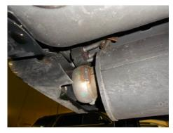
3) Once the factory system is out of the vehicle, use a 5/16 wrench to remove the three nuts securing the actuator to the mounts on the tailpipes. Remove the actuator and spring from the mount on each tailpipe.
