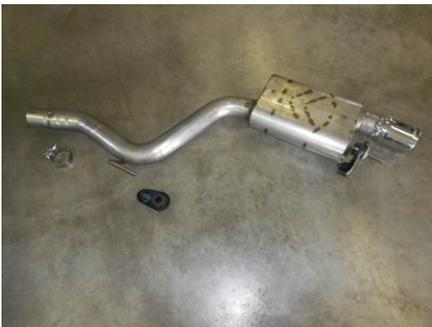
1) Place the new Flowmaster muffler units next to the factory units and swap the front and rear hanger mounts from the stock mufflers to the Flowmaster assemblies. Also, place a provided 2.25" clamp onto the inlet of each assembly. Tighten the clamp just enough to hold in place.
