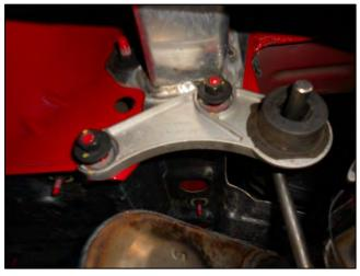
3) After cutting the two front pipes and with the factory muffler still supported, remove the two hangers at the front of the muffler from the rubber mounts on the vehicle. You can now lower the supports at the front of the muffler and slide the muffler forward to disengage the rear hangers from the mounts on the vehicle.
