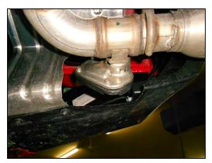
4) Lower the muffler slightly to gain access to the exhaust valves on both outer exit pipes and unplug the electrical connection from the actuator. Lower the muffler from the vehicle and place it next to the new Flowmaster mufflers. Carefully deburr the end of the pipes where cut with a file or die grinder. Then using a 15mm wrench, unbolt the two factory hangers at the rear of the vehicle from the frame and place them onto the new Flowmaster muffler assemblies.
