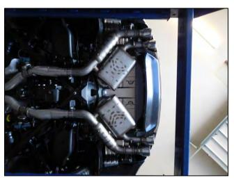
3) Adjust and level the two muffler assemblies to provide a satisfactory fit. They can also be adjusted forward or back to get the desired position in the rear valance cut-outs. A minimum of 1/2" clearance around all parts of the system must be maintained; while keeping suspension travel and vibration in mind. After adjustments have been made, and you are satisfied with the fit, you may now securely tighten the two muffler inlet clamps.
