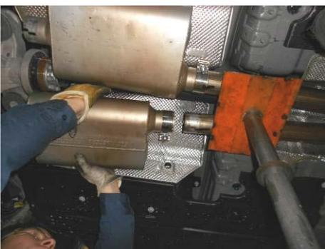
5) Place a supplied 2 1/2" clamp onto the inlet of each **#842546-Z** muffler. Then fully slide the mufflers onto the back of the Scavenger pipe assembly and support with stands. Level the mufflers and tighten the clamps enough to hold, but still allow for adjustment.
