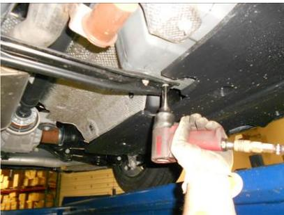
2) Using a 13mm socket, unbolt the two body braces in the center of the vehicle. The braces will be re-installed after completing step 2 of the installation instructions below.
