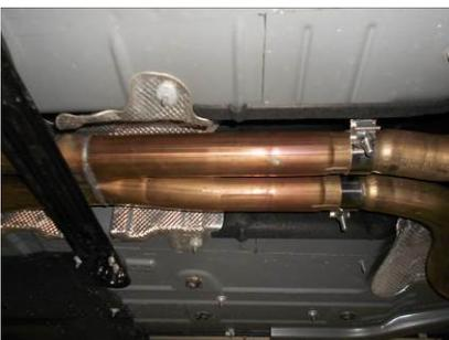
2) Begin by placing a supplied 2 1/4" clamp onto each of the slip fits on Scavenger pipe **#86331S**. Place the Scavenger pipe onto the back of the stock head pipes (make sure the Flowmaster embossing is facing the ground). Level and center the assembly in the drive line tunnel and support with a stand. Tighten the two clamps enough to hold, but still allow for adjustment. Reinstall the two body braces onto the vehicle and tighten securely.
