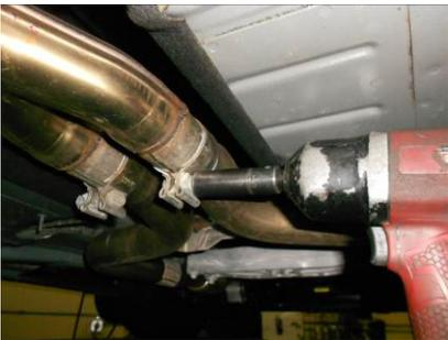
3) Support the rear of the system with a stand. Then starting at the rear of the vehicle, remove the hangers on the system from the rubber mounts on the vehicle, also un-clip the ground strap from the middle hanger on the right tailpipe. Then using a 15mm socket, loosen the clamps at the slip fit connections behind the catalytic converters and with the help of an assistant, lower the stand and slide the system back off of the head pipes. Carefully lower from the vehicle.
