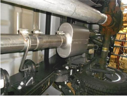
3) Slide the inlet hanger **#490HA** over the back of the inlet pipe and insert the hanger into the factory rubber mount. Do not tighten this clamp yet. If required, place the extension pipe **#26277S** onto the back of the inlet pipe. Then place the inlet of the muffler onto the back of inlet pipe and support with a stand. Level the muffler and tighten the clamp at the inlet enough to hold, but still allow for adjustment.
