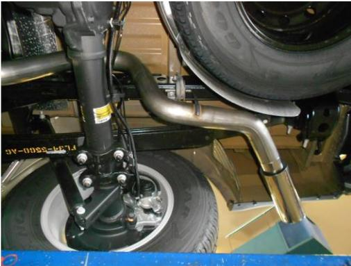
4) Install a provided clamp onto the muffler outlet. Then place tailpipe **#26575S** into position over the axle and into the muffler outlet while also connecting the hangers on the pipe to the rubber mounts on the vehicle. Tighten the band clamp enough to hold, but still allow for adjustment.
