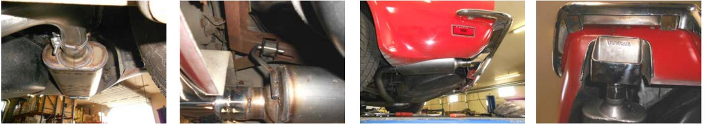
5) Adjust the position of the pipes and mufflers to provide a satisfactory fit. A minimum of 3/4" clearance around all parts of the system must be maintained; while also keeping suspension travel and vibration in mind. Tighten all clamped connections down securely.
