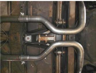
2) Place a provided clamp onto both outlets of X-pipe assembly **86233S**. Place the expanded end of mid pipe **86237S** onto the right outlet of the X-pipe assembly. Rotate the pipe up into position and support the rear of the pipe with a stand. Tighten the clamp enough to hold, but still allow for adjustment. Repeat this step on the left side of the vehicle with pipe **86238S**.
