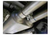
9) Install a provided 3" clamp onto the right muffler outlet. Place the right side tailpipe **#26465S** into position over the axle and slip into the right side muffler outlet, while at the same time, connecting the hangers at the front and rear of the pipe to the rubber mounts on the vehicle. Tighten the clamp enough to hold, but still allow for adjustment.
