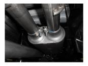
10) Install a provided 3" clamp onto the left muffler outlet. Place the front section of the left side tailpipe **#26466S** into the left side muffler outlet and connect the hanger on the pipe to the rubber mount on the vehicle. Tighten the clamp enough to hold, but still allow for adjustment. Place a second 3" onto the back of this pipe in preparation for the next step.
