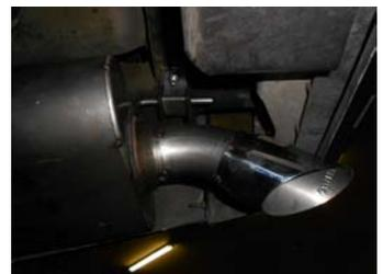
3) Place one of the supplied **HA602** rubber mounts onto the wire hanger of left muffler assembly **#842550-324**. Place the muffler assembly onto the back of the Y-pipe and slide the two pipes fully together, support the muffler with a stand. Using a supplied 3/8" bolt, nut, washer and lock washer, bolt the **HA602** hanger to the hole in the frame above the muffler outlet.
