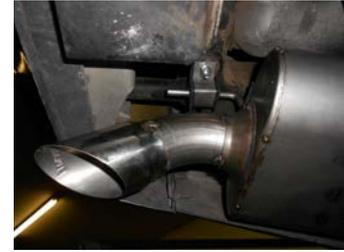
4) Adjust the position of the pipes and mufflers to provide a satisfactory fit. A minimum of 3/4" clearance around all parts of the system must be maintained; while also keeping suspension travel and vibration in mind. Tighten all clamped connections down securely.
