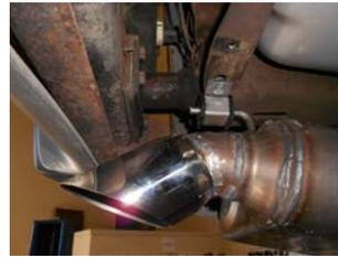
4) Adjust the position of the pipes and mufflers to provide a satisfactory fit. A minimum of 3/4" clearance around all parts of the system must be maintained; while also keeping suspension travel and vibration in mind. Tighten all clamped connections down securely.
