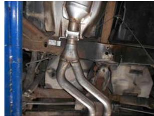
2) Place a provided clamp onto both outlets of Y-pipe assembly **#86105S**. Place one of the supplied **HA602** rubber mounts onto the wire hanger of right muffler assembly **#842554-321**. Place the muffler assembly onto the back of the Y-pipe and slide the two pipes full together, support the muffler with a stand. Using a supplied 3/8" bolt, nut, washer and lock washer, bolt the HA602 hanger to the hole in the frame above the muffler outlet.
