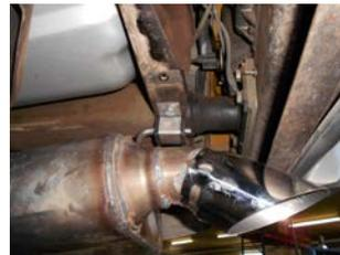
3) Place one of the supplied **HA602** rubber mounts onto the wire hanger of left muffler assembly **#842554-320**. Place the muffler assembly onto the back of the Y-pipe and slide the two pipes full together, support the muffler with a stand. Using a supplied 3/8" bolt, nut, washer and lock washer, bolt the HA602 hanger to the hole in the frame above the muffler outlet.
