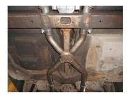
1) After installing either the **81095** or **81098** downpipe kits, place a provided 2.25" clamp onto the expanded ends of X-pipe assembly **86171S**, then slide onto the back of the manifold pipes, be sure that the pipes are fully slid together. Place a stand under the rear of the assembly and tighten the clamps enough to hold, but still allow for adjustment.
