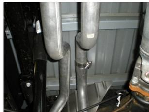
10) Connect the rear section of the left side tailpipe **#86034S** onto the back of the front section by sliding the two sections together at the slip-fit connection over the rear axle. Place the hanger at the rear of the tailpipe into the rubber mount installed in Step 6 above. Tighten the clamp enough to hold, but still allow for adjustment.
