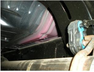
5) On Crew-cab long bed models, there are three hangers between the muffler and the catalytic converter, two with a rubber isolator and one without. Take the rubber isolator from the second hanger from the muffler and place it onto the hanger welded to the frame midway between the converter and the muffler. Slide clamp hanger **#459HA** over the back of inlet pipe **#26396S** and connect to this rubber mount.
