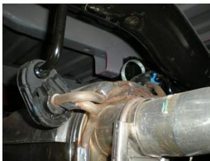
3) Support the muffler with a stand and remove the two hangers at the rear of the muffler along with the hangers in front of the muffler from the rubber mounts on the vehicle. Then remove the clamp on the slip connection just behind the catalytic converter. **After removing the clamp, this connection will need to be either sliced or heated in order to separate the connection.** Remove the muffler and set aside.
