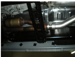
4) Trim inlet pipe **#26396S** according to the following measurements before placing onto the stock front pipe just behind the catalytic converter. Be sure to line up the notch in the pipe with the tab on the front pipe. Place the provided 3" clamp onto this connection and tighten enough to hold.
