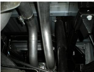
8) Install a provided 2½" clamp onto the right muffler outlet. Place the right side tailpipe **#86033S** into position over the axle and slip into the right side muffler outlet, while at the same time, connecting the hangers at the front and rear of the pipe to the rubber mounts on the vehicle. Tighten the clamp enough to hold, but still allow for adjustment.
