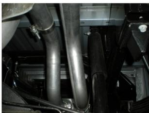
9) Install a provided 2½" clamp onto the left muffler outlet. Place the front section of the left side tailpipe **#86032S** into the left side muffler outlet and connect the hanger on the pipe to the rubber mount on the vehicle. Tighten the clamp enough to hold, but still allow for adjustment. Place a second 2½" onto the back of this pipe in preparation for the next step.
