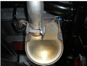
2) To make the removal of the stock system easier, using a hacksaw or sawsall cut the stock tailpipe off where it exits the muffler. Remove the hanger at the rear of the tailpipe from the rubber mount on the vehicle and set the tailpipe aside. This step is not mandatory, but makes removal easier. There are retainer clips on the ends of each of the hangers that will need to be removed with pliers to allow disassembly.
