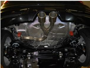
8) Place the two **#ST459** stainless tips onto the outlets of the exit pipe and adjust to the desired position. Tighten the clamp on the tips enough to hold, but still allow for adjustment.
