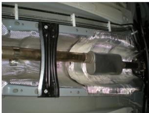
4) Using the 7/16" bolts, nuts and washers provided, bolt resonator assembly **15174S** to the back of the flex pipe flange. Be sure to replace the gasket. Support with a stand. Then reinstall the steel body brace removed in the previous step and tighten securely.
