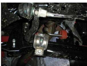
6) Place a supplied clamp onto the expanded end of over-axle pipe **#86010S** and slip it onto the back of pipe **#16738S**. Connect the hanger on the pipe to the rubber mount on the vehicle and tighten the clamp enough to hold, but still allow for adjustment.
