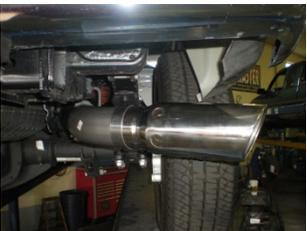
4) Place a supplied 4" clamp onto the expanded end of stainless tip **#ST475** and slide onto the end of the tailpipe and adjust to the desired location.
